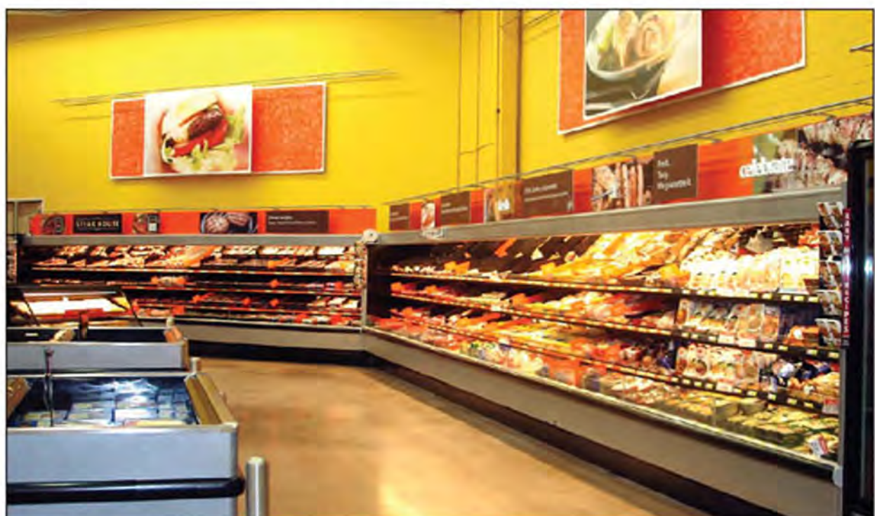
■ As part of Wal-Mart's commitment to building environmentally friendly stores, the Garner, N.C., Supercenter uses recycled materials in its concrete flooring and the floor's finish reduces the need for chemical cleaners.
