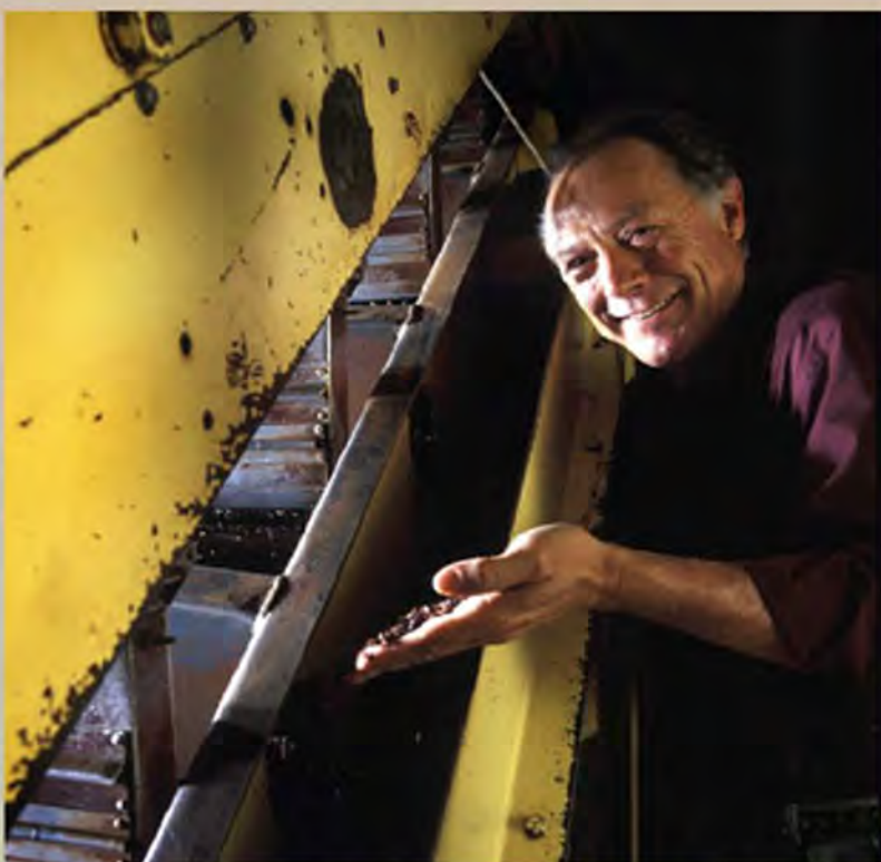
GARY GUITTARD with winnowing machine called the cracker fanner used to separate the shell from the cocoa beans which leaves the nibs to be ground into cocoa mass.
